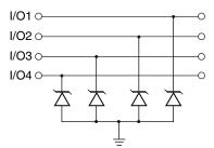
**Unidirection Protection of Four Lines**
